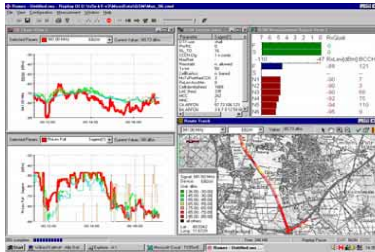
Special views combined with diagram and map view for convenient analysis: here GSM measurements
